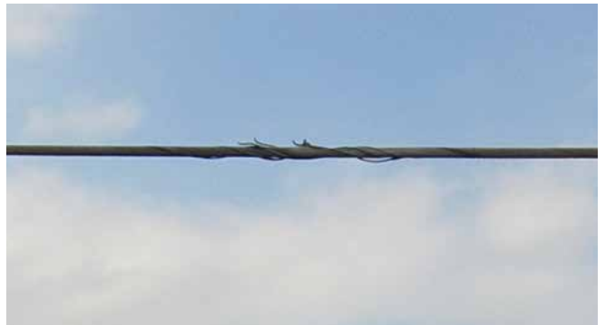
Conductor damage due to gun shots out of JC Hall substation
